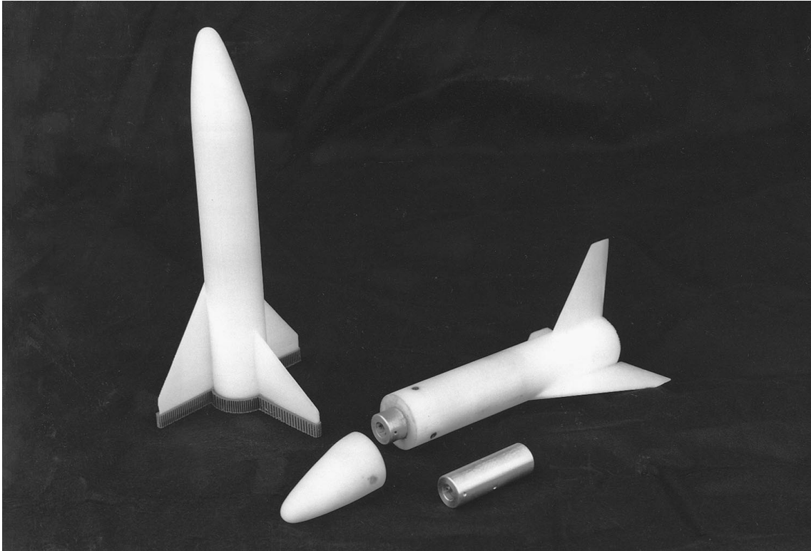
FIGURE 11.—Fused deposition method model straight from the machine, with fabrication stand, model converted into wind tunnel model, and aluminum balance adapter.
