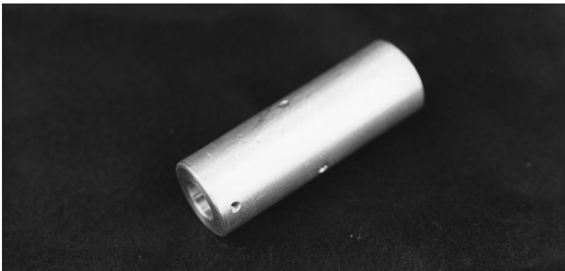
FIGURE 12.—Aluminum balance adapter used in models.
