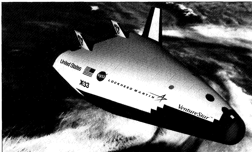
X-33 Advanced Technology Demonstrator designed to demonstrate in flight the new technologies needed for a Reusable Launch Vehicle for the 21st century. The X-33 employs a lifting-body shape. (NASA photo EC96 43631-2)
