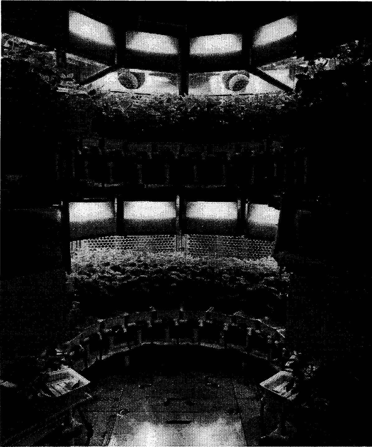
FIGURE 2. Soybean plants (cv. McCall) growing in the upper half of NASA's Biomass Production Chamber. Plants were grown in plastic culture trays using nutrient film technique. Trays were supported on four vertically-stacked shelves (two shown in the photo) with 16 trays per shelf, providing a total of 20 m 2 of growing area. Lighting was provided by high-pressure sodium lamps in the upper half of the chamber and by metal halide lamps in the lower half of the chamber.
