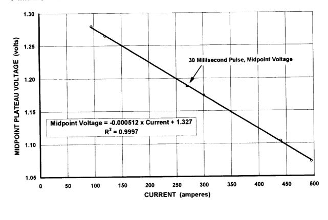
Midpoint plateau voltage data obtained at high states of charge are summarized in the plateau voltage *versus* pulse current chart. The slope of the voltage *versus* current plot is the cell resistance; the linear relationship is an expression of Ohms Law.
