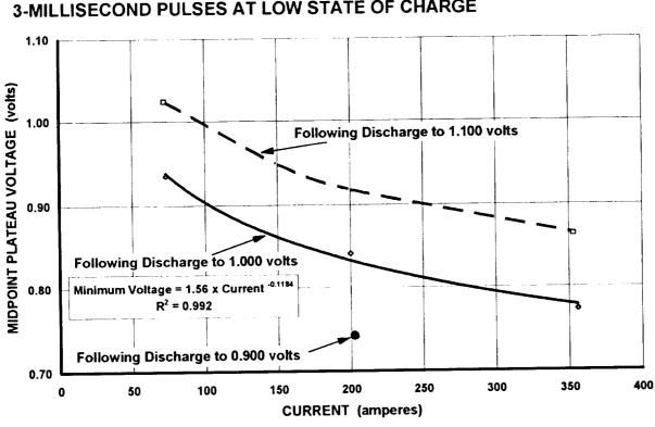
AVERAGE MINIMUM VOLTAGE 3-MILLISECOND PULSES AT LOW STATE OF CHARGE
