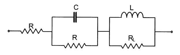
Cell performance can be described by simple equivalent circuits for the simulated fault clearing events presented here. A complete description of cell impedance includes inductive, resistive, and capacitive elements. as well as terms dealing with electrochemical phenomena. A "complete" cell equivalent circuit would contain all these elements and would be very complex. However, in the time domain, and at the operating conditions studied, significant simplifying assumptions are possible.
