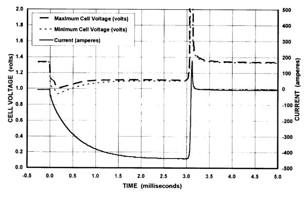
The 450-ampere discharge also shows excellent voltage "stiffness" during the fault clearing discharge. The difference between the starting voltage, e.g., the voltage prior to the fault clearing event, and the plateau voltage is greater than observed with the 150 ampere discharge. As will be seen in the succeeding charts the relationship between the initial and plateau voltages is a function of cell impedance and follows Ohms Law.
