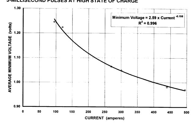
The minimum voltage observed during the fault clearing event may be of interest in terms of spacecraft bus voltage regulation. This chart shows the relationship between the average minimum voltage and the pulse current for the fault clearing data obtained at high state of charge.
