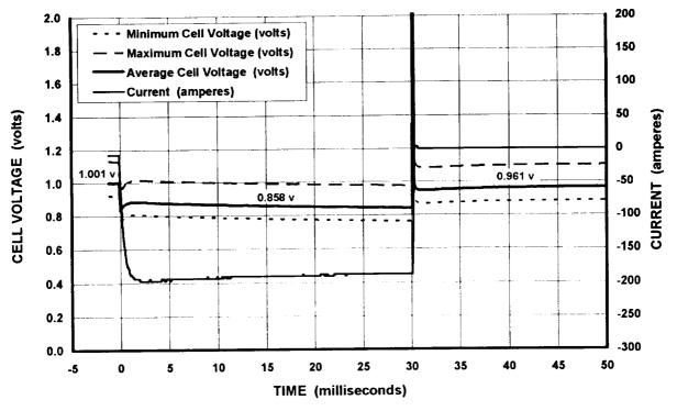
Thirty-millisecond pulse data, at low state of charge, is shown to demonstrate that the plateau voltage trajectory exhibits a negative slope as energy is removed. This slope, plus the lower post fault clearing voltage, is interpreted as indicating that the cell capacitance is changing significantly, in this time domain, at these operating conditions.
