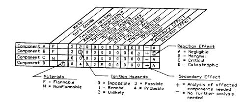
Figure 2 Oxygen Hazards Analysis Chart.
