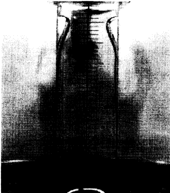
Figure 5: Videoprint of a subcritical flow between two parallel plates. The optical axis is perpendicular to the plates, the flow is from the bottom to the top (same parameter as Fig. 4).
