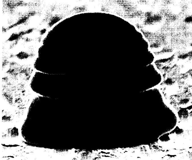
Figure 3: Solder microbump obtained experimentally in normal gravity. The solidified bump was produced by the deposition of a single 50 \mu\text{m} -diameter droplet.
