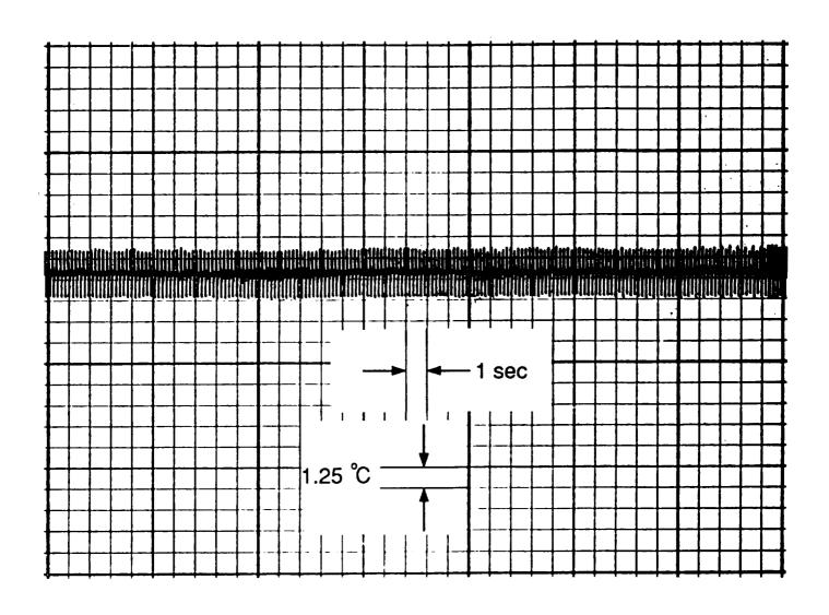
Fig. 2 Temperature oscillation detected in a tin liquid bridge.
