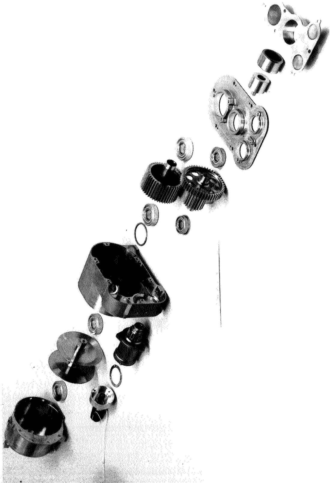
**Figure 8 Airbag Retraction Actuator Exploded View**
