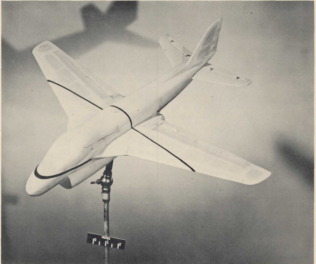
Figure 3.- Photograph of 1/28-scale model of the test airplane in the clean condition with the original tail configuration. L-59-3857
