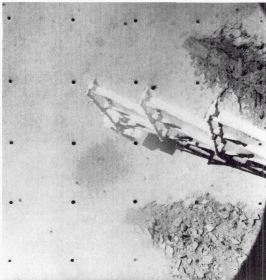
Surveyor surface sampler pauses between two trenches it dug in lunar material.
