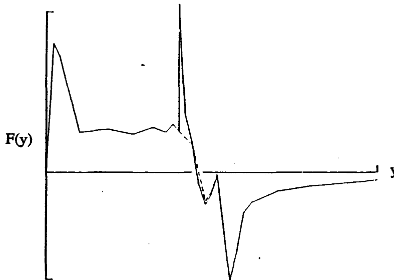
Figure 7. Combined F-function computed from fuselage, wing, wing lift, fin, and interference lift equivalent areas. (The dashed lines show the original lines in figure 6.)
