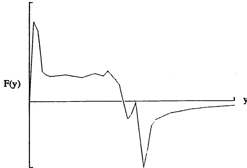
Figure 3. Typical F-function computed from equivalent areas in figure 2.
