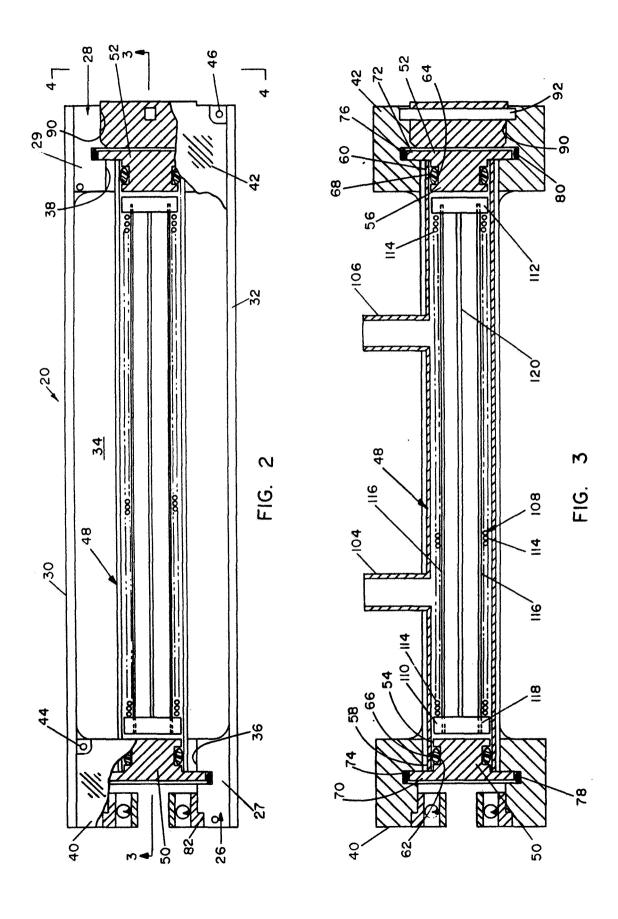
shown) are powered by a rotating shaft of the motor 14. Thus it can be seen that rotation of the drive shaft 22 causes rotation of the culture vessel assembly 20 through the action of the key members extending from the drive member 96.
