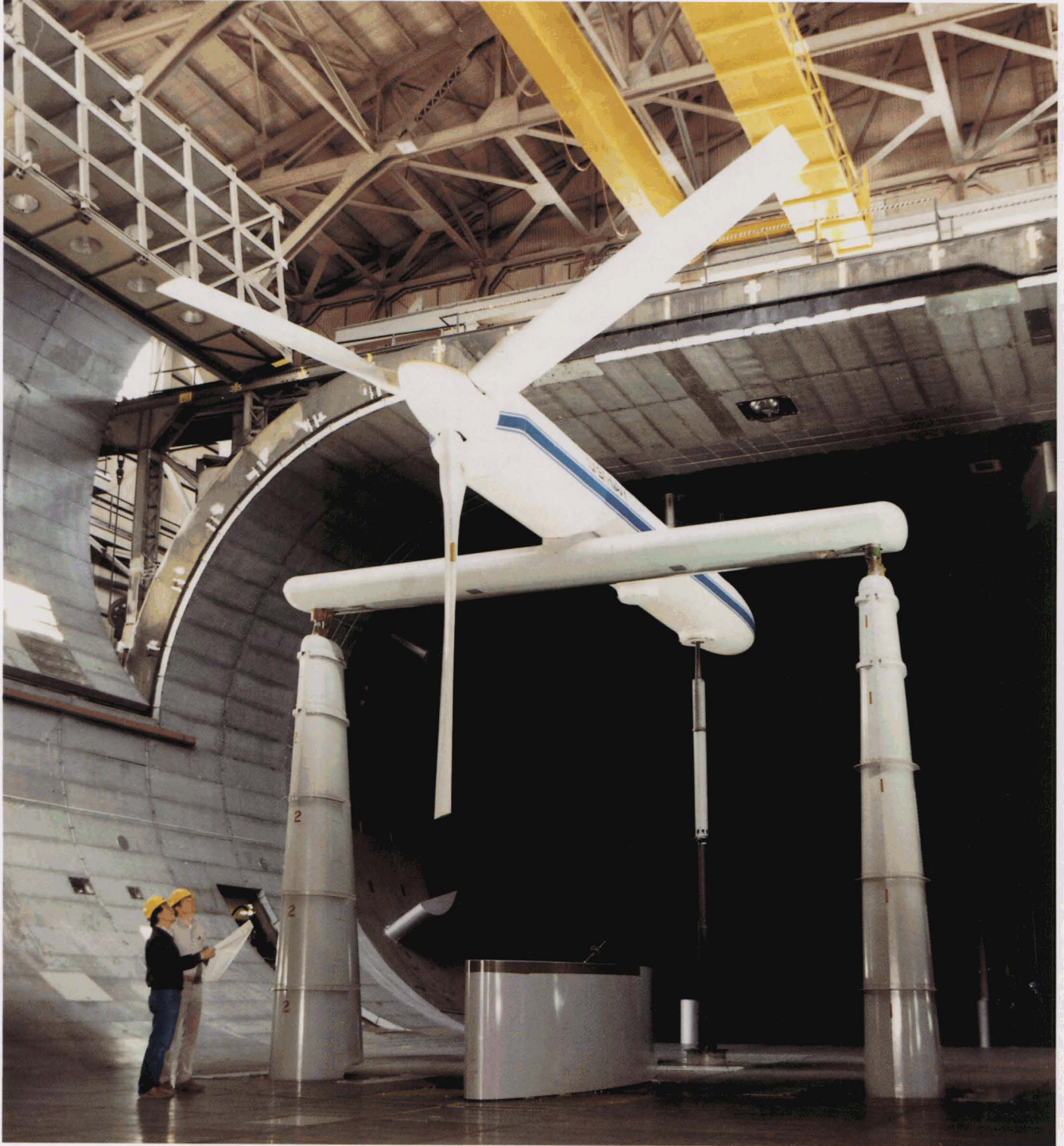
Large Scale V-22 Rotor Tests in 40 by 80 ft. Wind Tunnel
