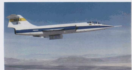
F-104 Aircraft with Flight Test Fixture Installed
