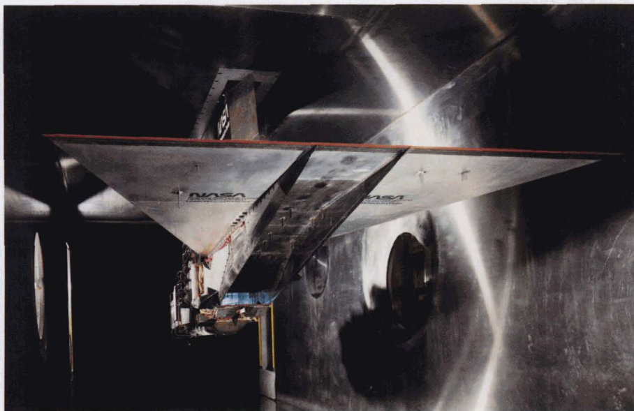
Hypersonic Inlet Under Test for Validation of CFD Analytical Codes
