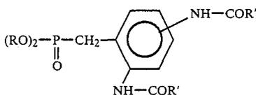
wherein R is a non nitratable organo group selected from alkyl groups having 1 to 10 carbon atoms, a group where the two R groups together form a single bridging alkylene having from 3 to 6 carbon atoms, halogen substituted alkyls having from 1 to 10 carbon atoms, R' is selected from alkyls having from 1 to 8 carbon atoms or phenyl, and the two amidos are in the 2,4 or 2,6 positions.
