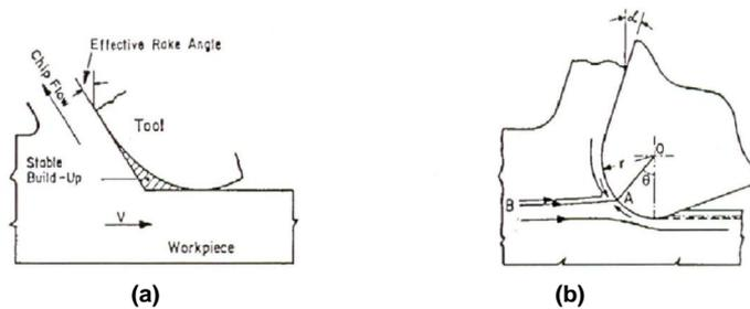
Figure 1: (a) A stable built-up edge during machining with blunt tools, (b) The metal flow around a rounded tool edge (Basuray et al (1977))
