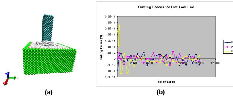
Figure 6: (a) Simulation with flat end tool, (b) Cutting forces for depth of cut of 5 Angstroms
