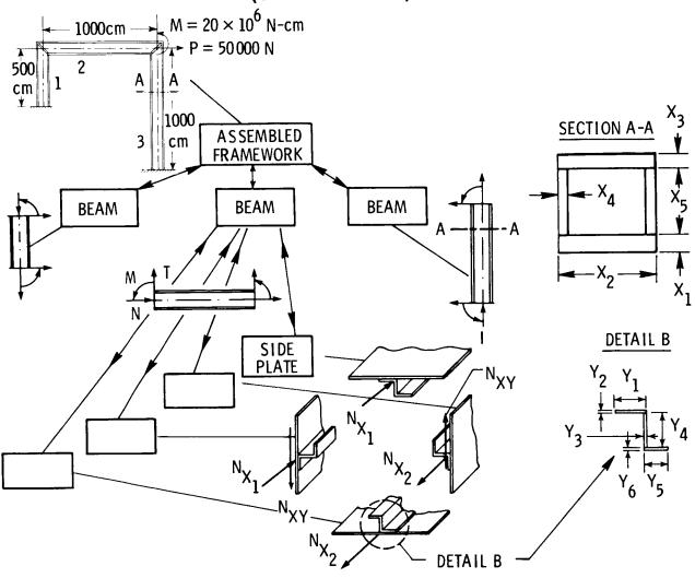
This is a summary of multilevel structural optimization development and testing. The method was also applied in a test case of a high-performance sailplane wing design (ref. 5). The results obtained to date are encouraging.
