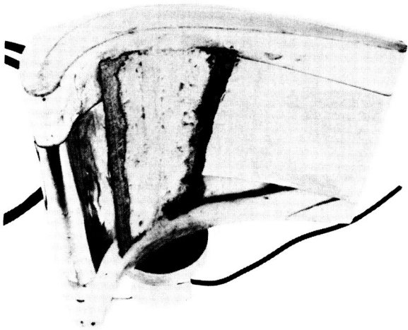
AIRFOIL WITH INSTRUMENTATION CAVITY CLOSED
