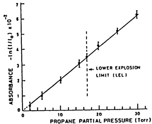
Fig. 4 Measured dependence of the absorbance at 1.6837  $\mu\text{m}$  on  $\text{C}_3\text{H}_8$  partial pressure in 1 atm.  $\text{C}_3\text{H}_8$ -air mixture contained in a 50-cm-long gas sensor head using a 2-km-long very low-loss silica optical fiber link.
