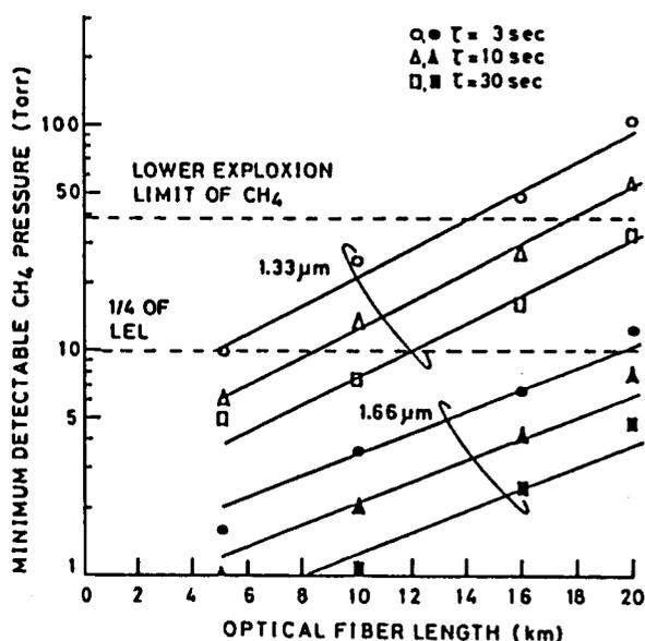
Fig. 3 Minimum detectable pressure of  $\text{CH}_4$  gas in air at 1.331 and 1.666  $\mu\text{m}$  as a function of the optical fiber length and the detection time in the all-optical remote measurement employing 5 - 20 km-long ultralow-loss silica optical fiber links in conjunction with InGaAsP LED's and a 50-cm-long absorption cell as the gas sensor head.
