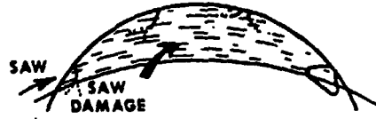
B. SLICING PUTS IN SAW DAMAGE AND CHIPS OUT SOME GRINDING CAVITIES.
