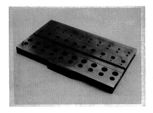
The flat plate specimens were used to continue testing of filler materials which survived the screening evaluation. This configuration, which is more representative of an actual model, incorporated coverplates with deliberate gaps around the perimeter, surface grooves, and various fasteners with submerged heads. The specimen was filled, measured, thermally cycled, and remeasured in the same manner as the screening specimens.
