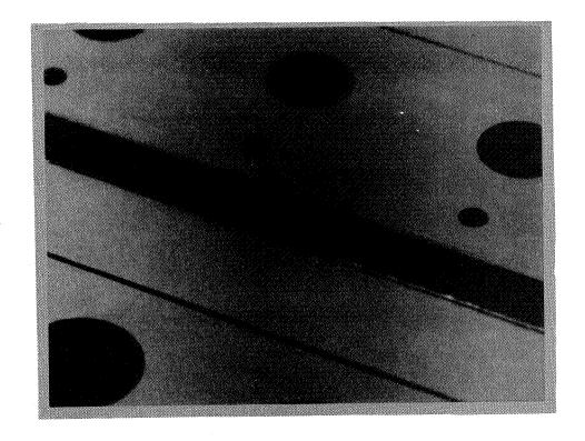
The bond line fractured and the filler material moved with respect to the metal surface during the thermal cycling. This type of failure was quite common, but seldom as dramatic as in this specimen. Failures of this type are attributed to stresses created by the mismatch of coefficients of thermal expansion between the metal plate and the filler material and the resultant relative contraction.
