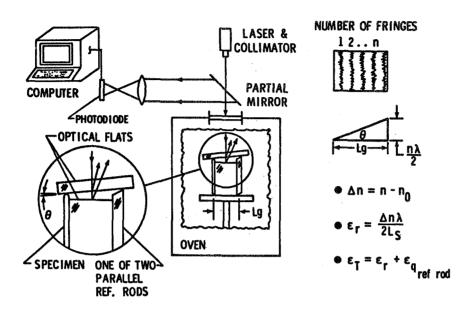
After experiencing several disappointments with the flat plate specimens which were related to mismatched coefficients of thermal expansion, it became obvious that the coefficients of the various candidate filler materials needed to be determined. The information generated would assist in matching filler materials to substrate metal, eliminating various fillers from further consideration, and determining optimum epoxy-to-filler ratios.
