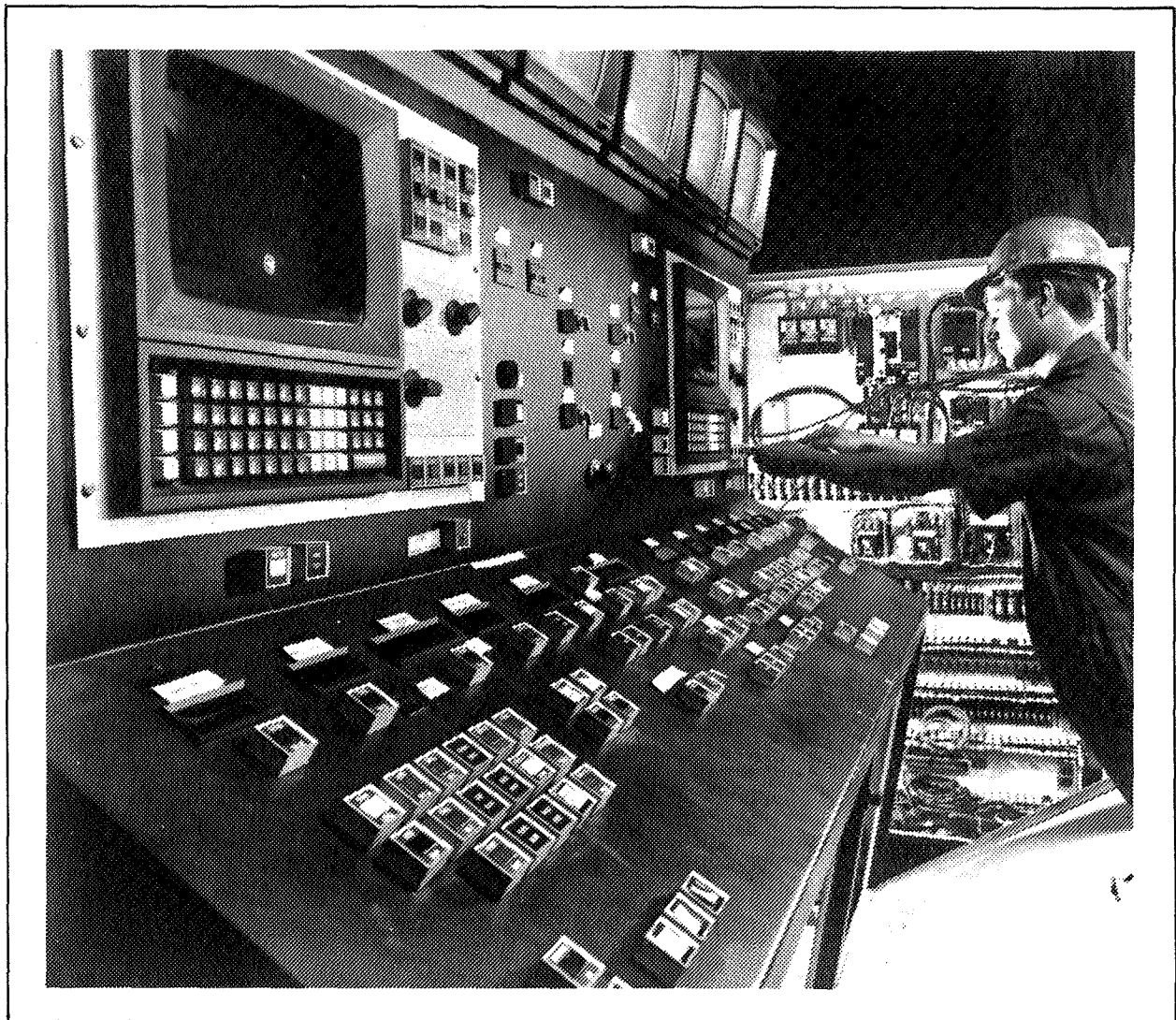
Figure 8. Operator's Console Provides Independent Control of Dual Drill/Riveting Systems.
