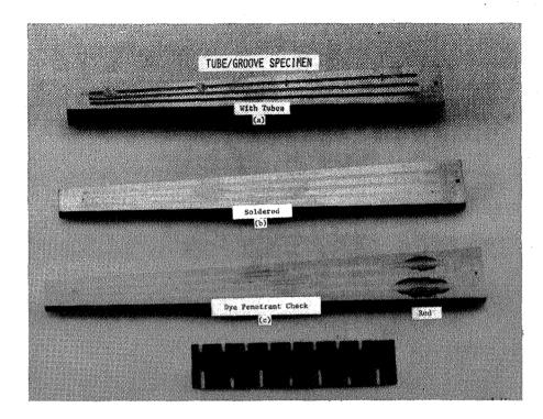
Now that a method of removing heat treatment oxides has been found, tube/groove specimens have been fabricated. The purpose of these specimens was to develop a method for soldering tubes in surface grooves. The specimens were then subjected to cryogenic temperatures.
