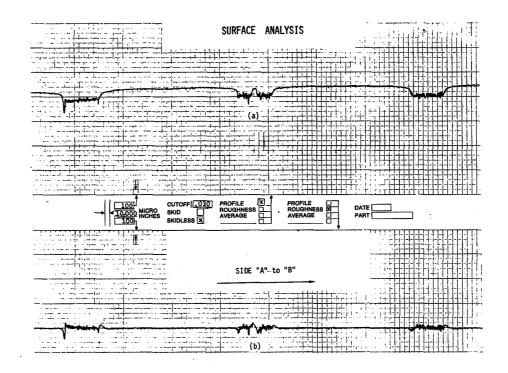
A surface analysis of the previous tube/groove specimen was done before and after cryo cycling. One cross section of the analysis is shown above. Solder at each groove has been undercut during finishing. The center groove of (a) has a raised spot in the middle because the tube was not on the groove bottom when soldered.
