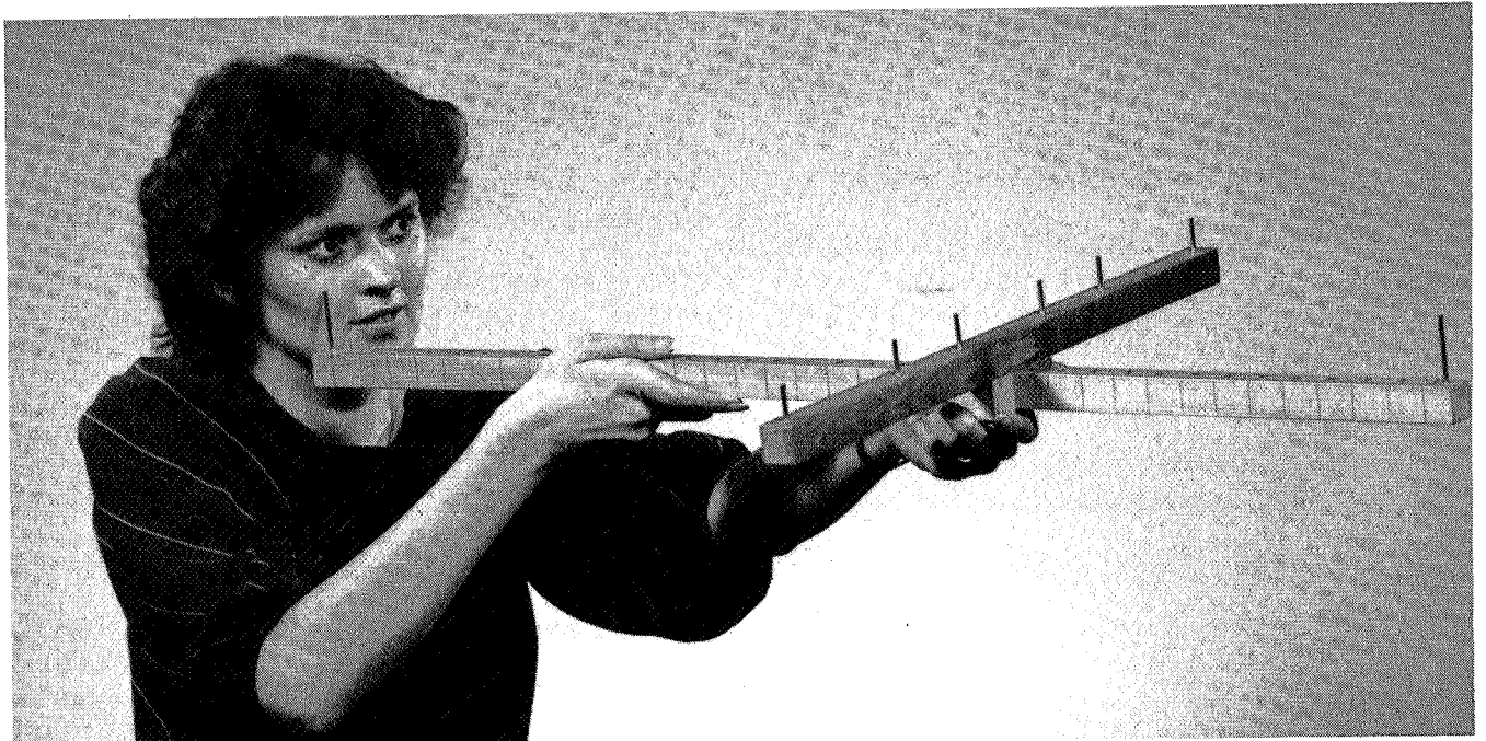
Aim the cross staff at the head and tail of the comet to determine the angular measurement of Comet Halley.
