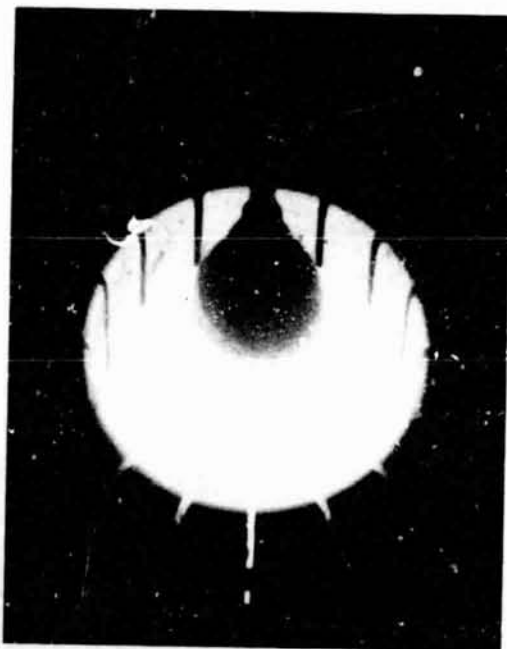
Dislocation-free silicon crystal being pulled from a cold crucible
