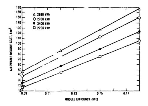
Energy Cost vs Module Cost and Efficiency, \$/kWh
