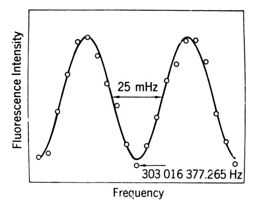
FIG. 2. Signal obtained with two 0.5s Ramsey pulses separated by a 19 s free precision interval on the clock transition in  $^{9}\text{Be}^{+}$  (see text). The sweep width was 100 mHz and the frequency interval between points was 5 mHz. The dots are experimental and are the average of 10 sweeps; the curve is a least squares fit.
