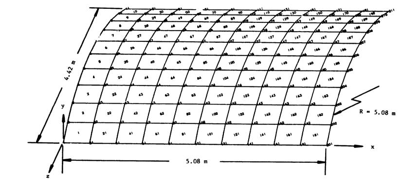
FIGURE 1 - SYMMETRIC LAMINATED COMPOSITE SHELL WITH [-60/0/60]35
