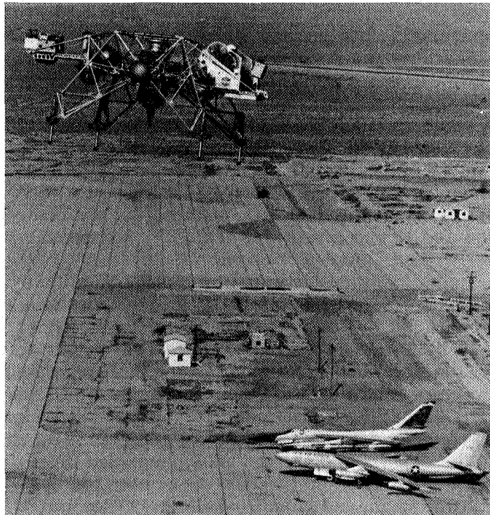
Joseph Walker pilots the first lunar landing research vehicle (LLRV) during tests at Edwards' South Base.
