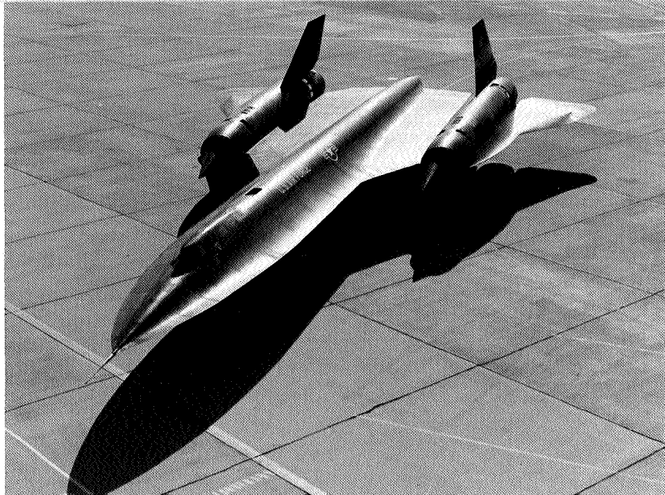
A low sun angle highlights the blended wing-body configuration of NASA's mach 3+ YF-12C Blackbird.
