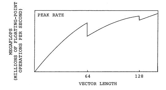
Figure 3. Vector processing on the CRAY
