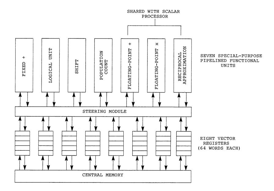
Figure 2. Vector processor of a CRAY computer
