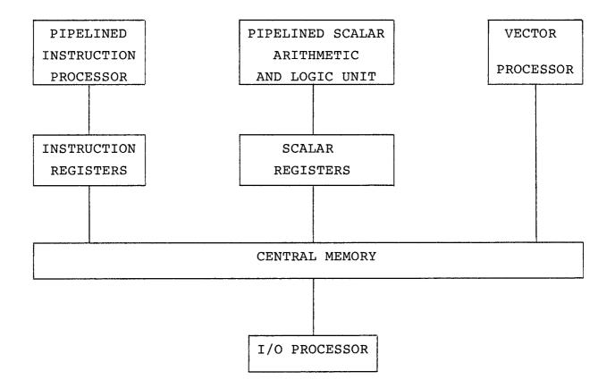
Figure 1. Generalized block diagram of a vector computer
