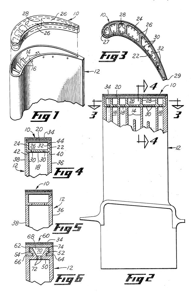
Another object of the present invention is to provide a replaceable tip cap with increased wear resistance
