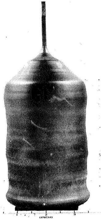
Figure 2. A 3.6 Kg, 3-inch Diameter, (100) LEC GaAs Crystal with Diameter Variation Less Than \pm 2\text{mm} .
