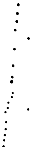
Figure 7. Stream of charged drops and one uncharged pair falling between high voltage plates.
