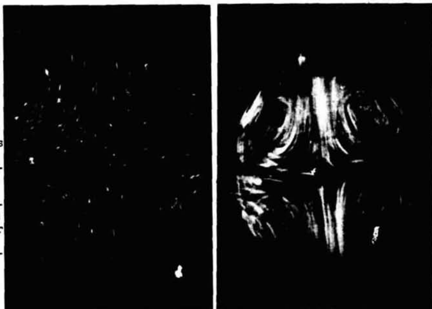
Figure 9: A. Streak patterns of suspended dye particles in a Silicone oil drop undergoing small amplitude oscillation in the L=2 mode. The drop is levitated in distilled water. ( \Delta R/R \leq 0.05 ) B. Streak patterns for the same drop oscillating at higher amplitude. ( \Delta R/R \approx 0.1 ).
