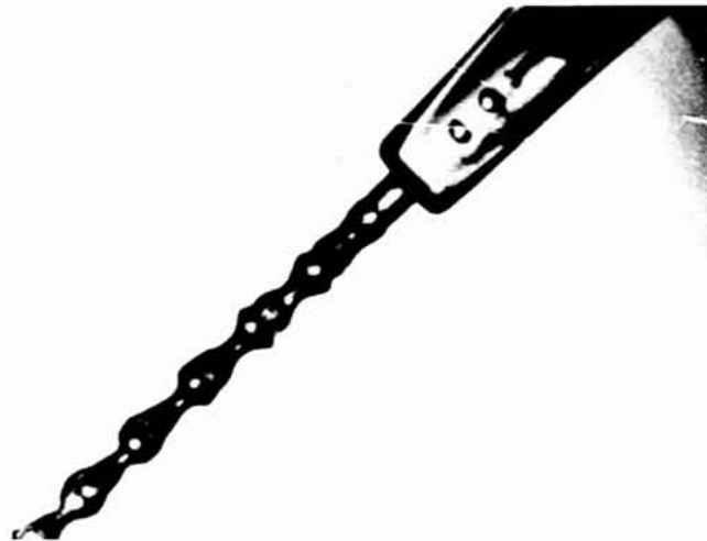
Figure 2 A water-air jet from which hollow spheres of water are being generated. The inner orifice can be moved axially to optimize the shell production. Gas flow rate, liquid flow rate, orifice diameters and drive frequency are important parameters. (1974)
