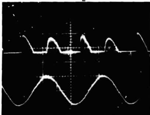
Fig.10. Scope trace of ac full-wave rectified current. Cd-Br boracite coplanar trielectrode sample with electrode spacing = 0.20mm; R_L = 100\Omega , R_p = 100K\Omega ; C_{bI} , C_{bII} = 10\mu F ; V_{dc} = 15V ; and temp = 301^\circ \pm 2^\circ C . Ac rectified current (upper trace): 0.1V/div. Applied 50 Hz ac voltage (lower trace): 0.5V/div. Time: 5 msec/div.
