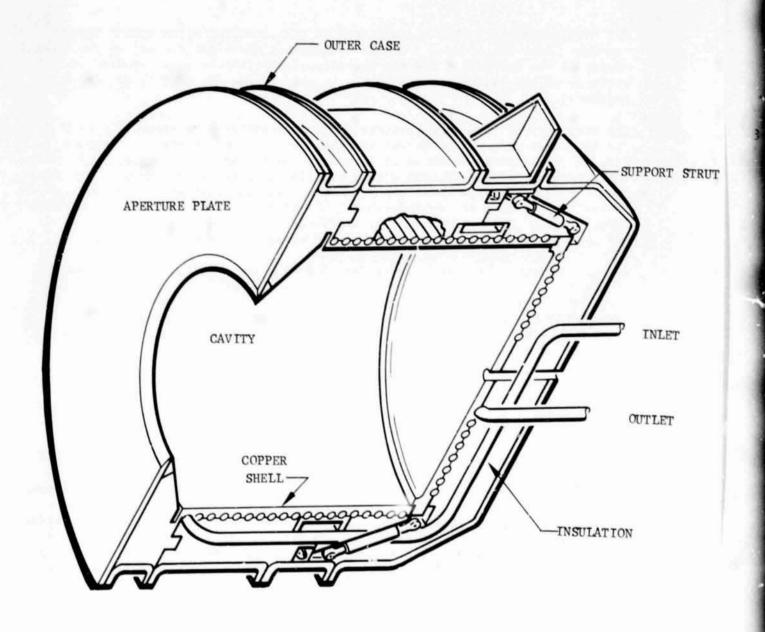
FIGURE 1. CUT-AWAY VIEW OF RECEIVER ASSEMBLY
