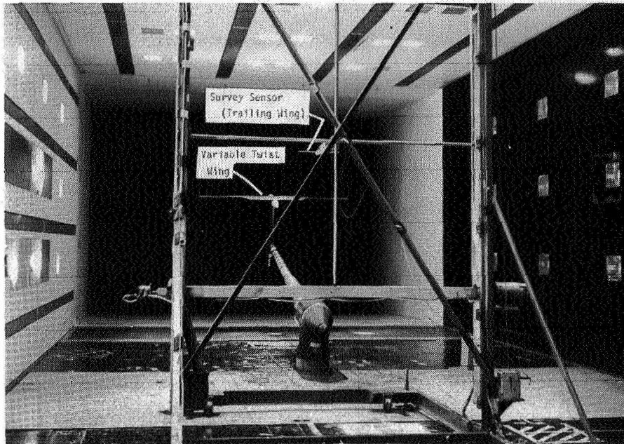
Figure 1.- Survey rig in Langley V/STOL Tunnel (with trailing-wing model attached to traverse mechanism.)
