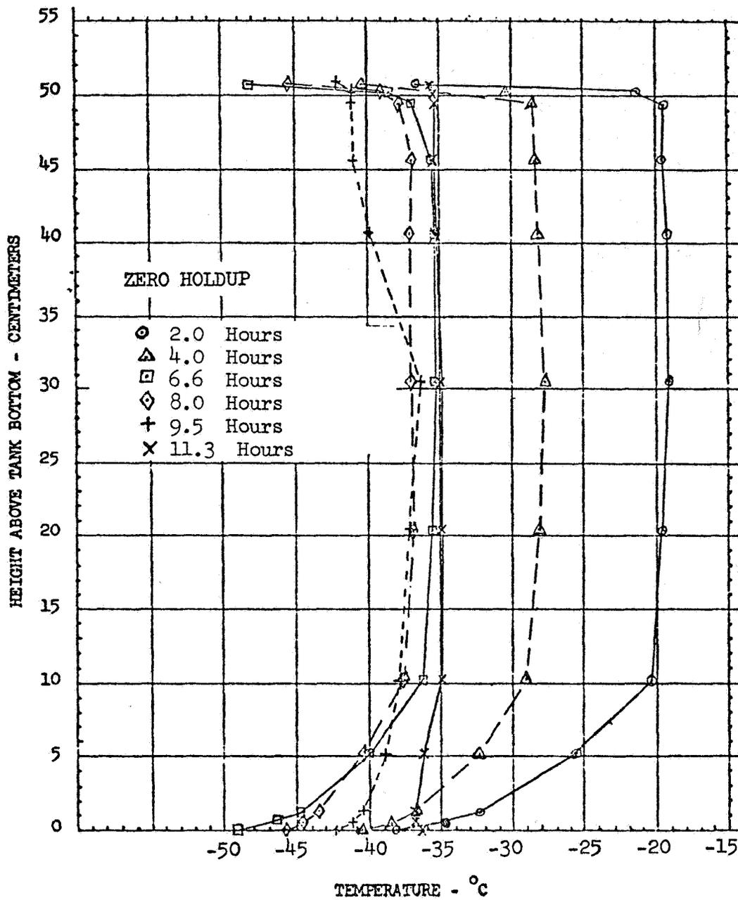
Figure - 6 Temperature Profiles at Center of Tank, Test 94
