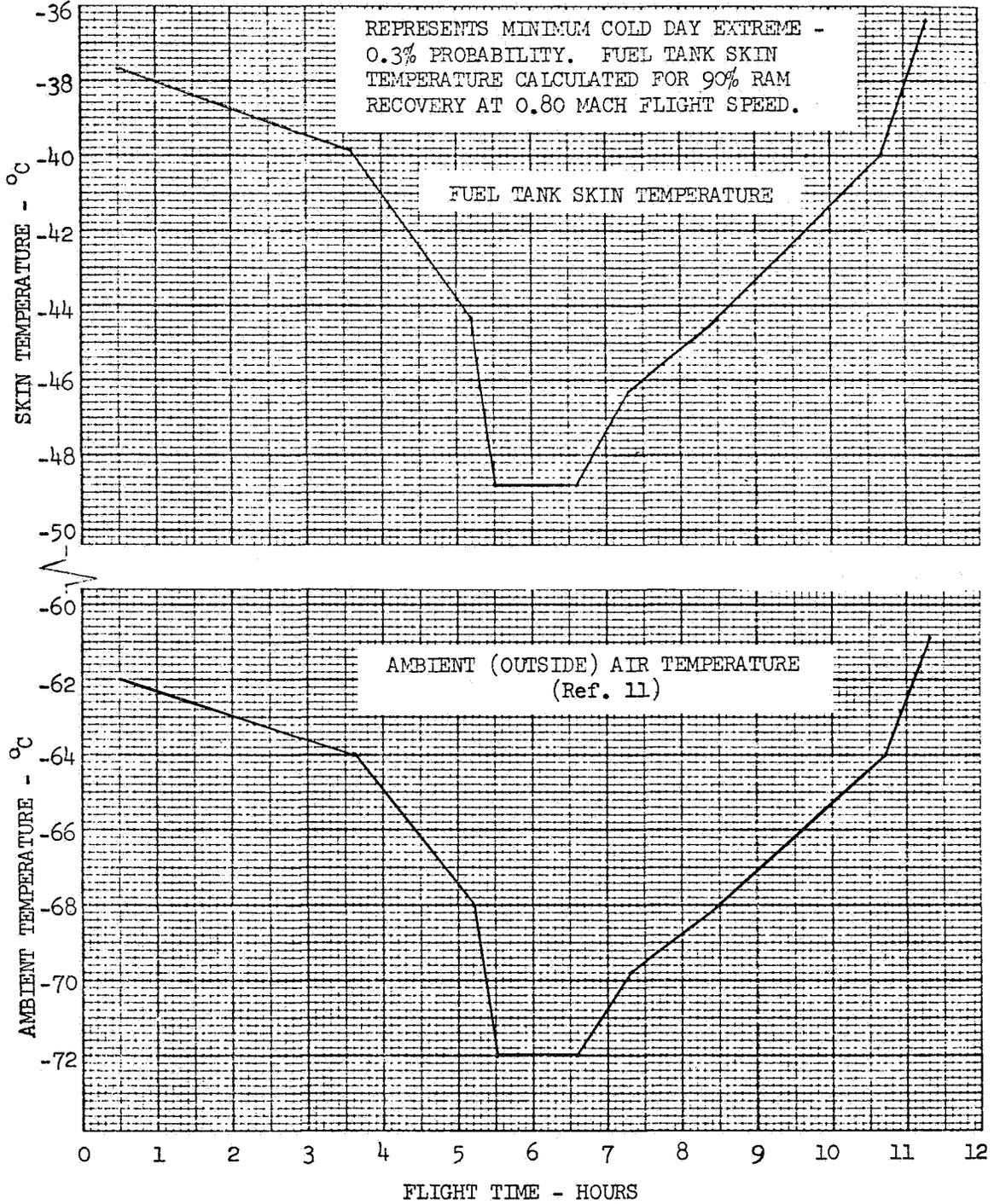
Figure - 5 Temperature Schedule for Scheduled Withdrawal Tests
