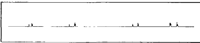
Figure 6. Example of LSF after traversing an optically degraded flow field 5 cm aperture.
