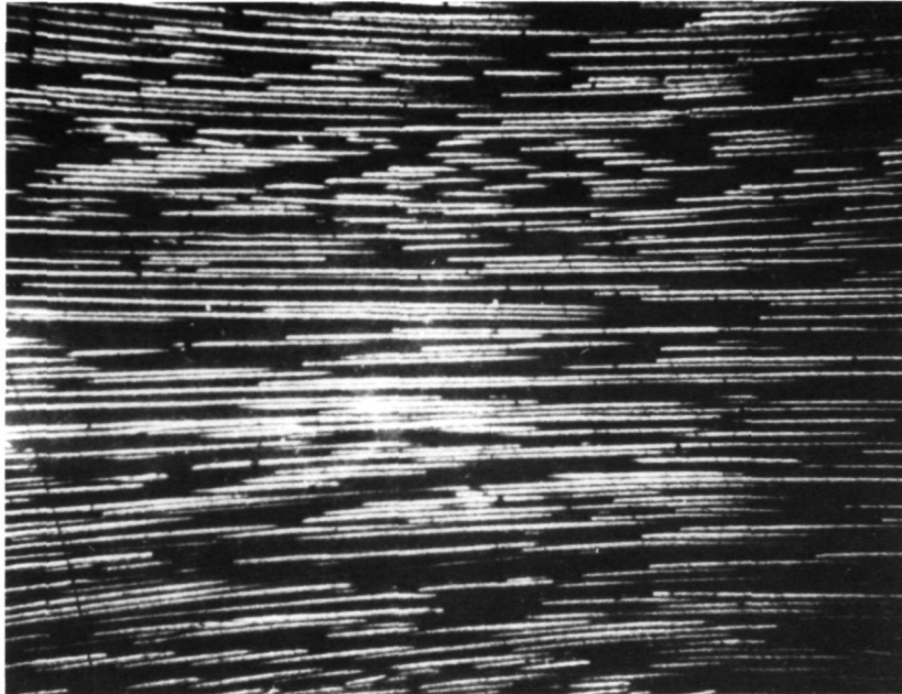
Figure 6.3 Lithium fluoride fibers in eutectic from the MA-131 Experiment. The cut-through bar of salt (enlarged 56 times) shows parallel fibers lined up by directional cooling from the molten state in zero-g.
