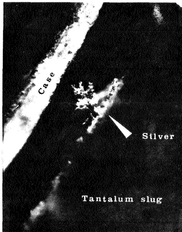
Figure 4. Type of growth that will result from application of reverse voltage (enlarged cross sectional view).
