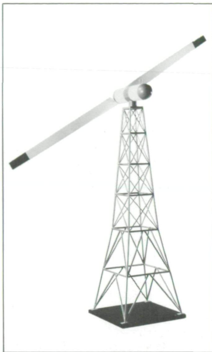
Model of 100-kilowatt windmill to be tested in Ohio. Rotor blades span 47.5 meters (125 feet) from tip to tip.
