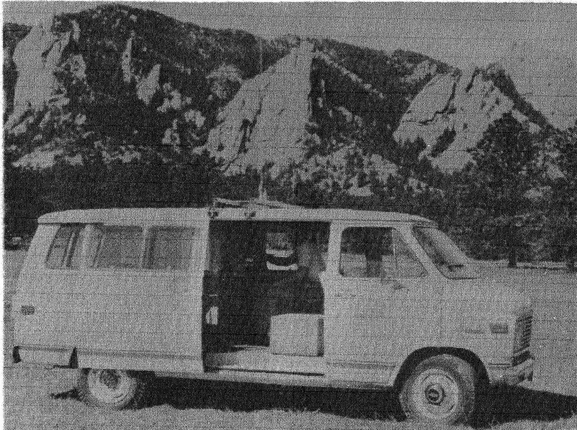
Figure 6. Vehicle housing modern Loran-C equipment capable of measuring both direct propagation time ( U ) and time difference ( y ) for calibration purposes.
