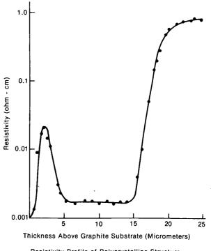
Resistivity Profile of Polycrystalline Structure
