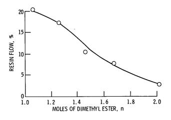
20% can be achieved. Moreover, the higher flow value PMR resins have use temperatures up to 561 K ( $550^{\circ}$ F), which is nearly 366 K ( $200^{\circ}$ F) above the use temperature for epoxies. For example, after 600 hours exposure at 561 K ( $550^{\circ}$ F), graphite fiber reinforced laminates made from these high flow PMR polyimides exhibited excellent strength and weight retention (70-78% strength retention and less than 4% composite weight loss).
