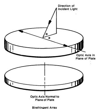
The birefringent retardation  $\Gamma$  is a function of the angles  $\Theta$  and  $\Phi$  that specify the direction of the incident light. A general expression for such a function is
