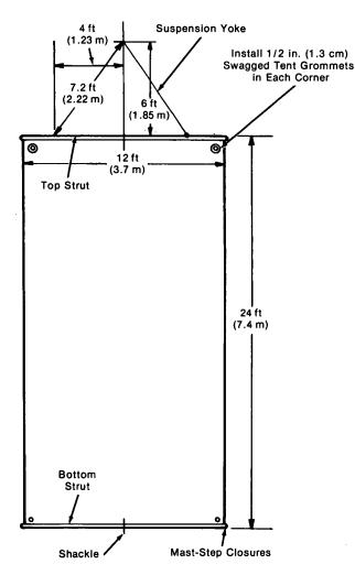
Note: Ballast weights are installed inside bottom strut and are contained with mast-step closures.
