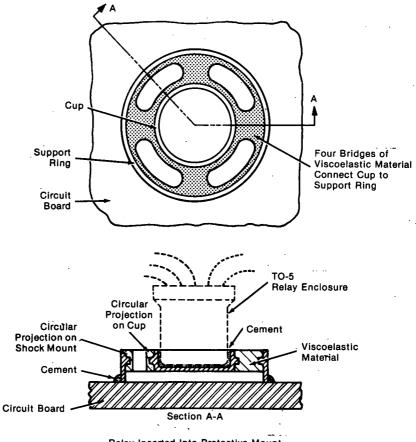
**Relay Inserted Into Protective Mount**
