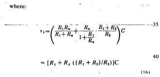
Equation 15 demonstrates that the effect of the finite 45 input impedance R, is to reduce the filter gain by a factor 1/K and to reduce the filter lag by the same factor. Consequently, the finite input impedance  $R_r$  must be taken into consideration in the design of the filter.
